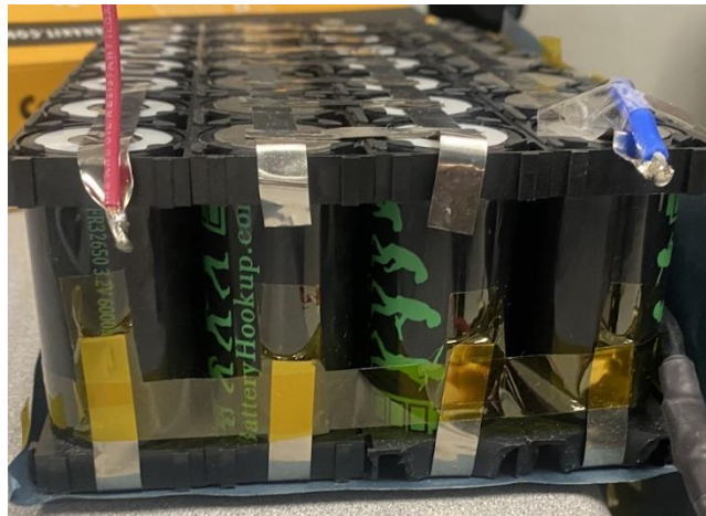
Figure A2. LiFePO4 Battery [52]
